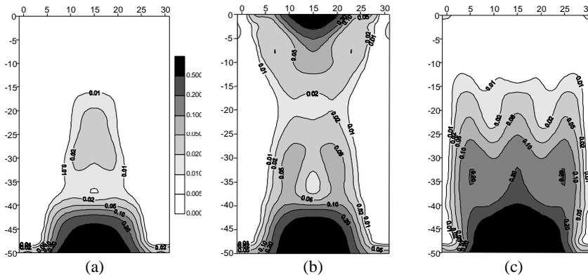
Fig. 4 Spatial distribution of Lagrangian multipliers derived from the spread function distribution shown in Figure 2; (a) cross-hole, inline and hole-to-surface data, (b) cross-hole and inline data, and (c) cross-hole and hole-to-surface data.
