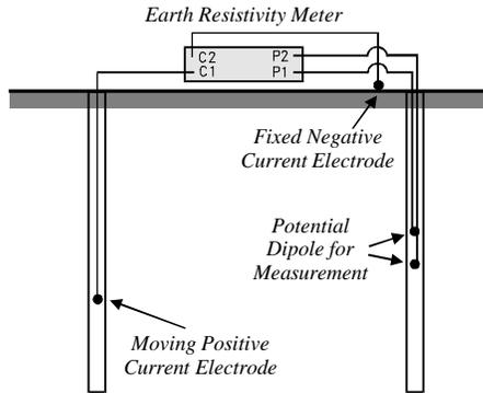
Fig. 2 A schematic presentation of the modified pole-dipole array for resistivity tomography measurement.
