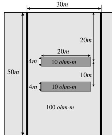
Fig. 1 Synthetic model used in the resistivity tomography. Two conductive objects are present at the center of the section.
