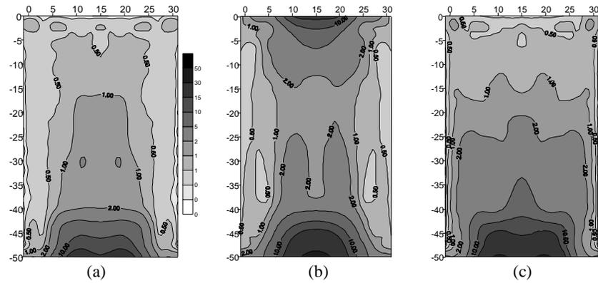
Fig. 3 Spatial distribution of spread function, based on the model of 100 ohm-m half space for different data sets; (a) cross-hole, inline and hole-to-surface data, (b) cross-hole and inline data, and (c) cross-hole and hole-to-surface data.
