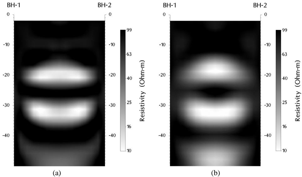
Fig. 5 Tomographic images (a) by the full optimization of the Lagrangian multiplier distribution through the Active Constraint Balancing, and (b) by a fixed Lagrangian multiplier of 0.05, a conventional approach. Data set configuration (a) in Figures 3 and 4 was used in the inversion.
