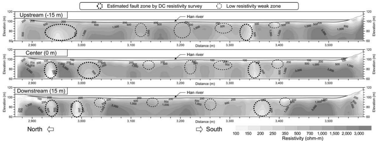
**Figure 6.** Three subsurface resistivity images obtained by water bottom installing method. The interpreted low resistivity weak-zones are superimposed on the inversion image as dashed circle.
