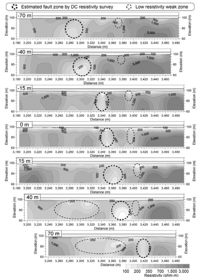
**Figure 8.** Comparison of inverted DC resistivity images of water bottom installing method (-15, 0 and 15 m) and streamer DC resistivity survey (-70, -40, 40 and 70 m). The survey lines of these images are parallel to the planned tunnel route with some apart to upstream or downstream side and located at south part of survey area.
