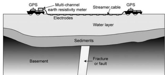
**Figure 7.** Schematic diagram of the layout of streamer DC resistivity survey at water-covered area. GPS is mounted on the vessel to provide the exact location of electrodes for each measuring moment. The streamer cable contains 19 electrodes with even 5 m spacing and it is towed by vessel.
