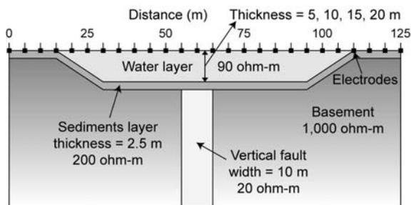
**Figure 1.** A schematic diagram of the numerical model of the DC resistivity survey at the water-covered area.
