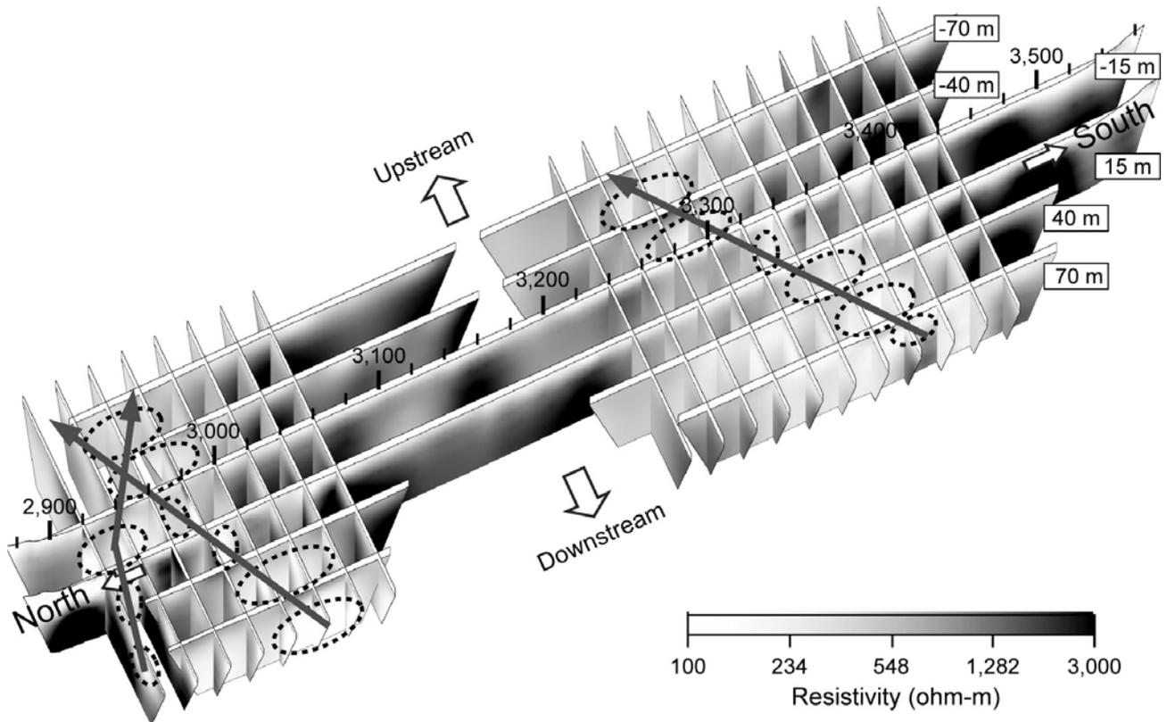
**Figure 9.** Three-dimensional fence diagram made by streamer DC resistivity images. The central two ones are obtained from water bottom installing method. It clearly shows the range and direction of three distinctive weak anomalous zones.
