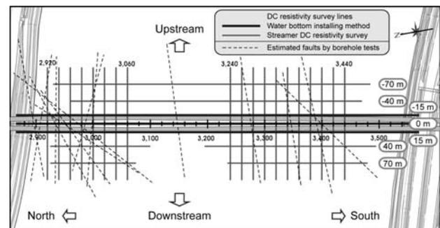
**Figure 5.** Location map of DC resistivity survey at Han River in Seoul, Korea. There are 7 parallel lines and 19 orthogonal ones to the planned tunnel route. Water bottom installing method is applied to central three bold lines, while streamer DC resistivity survey is applied to the others.
