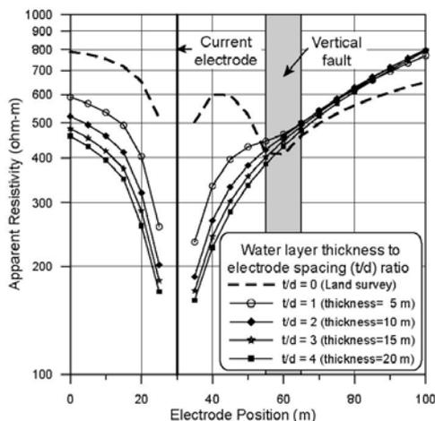
**Figure 4.** Variation of apparent resistivity along the profile line depending on the change of water layer thickness. The pole-pole array is deployed and electrodes are floated on the water surface with 5 m spacing. Current electrode and vertical fault are located at the position of 30 m and 55 ~ 65 m, respectively.
